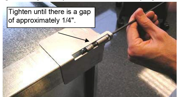
Figure 47: Tighten Cap Screw to 1/4" of the Coupling
